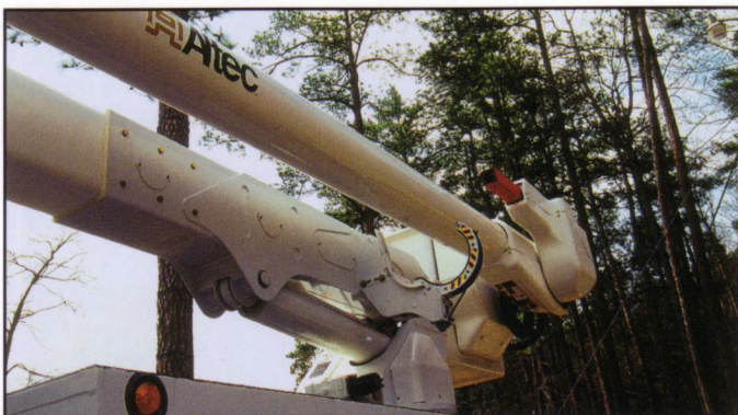
Automatic upper boom stow system reduces setup and stow times.
