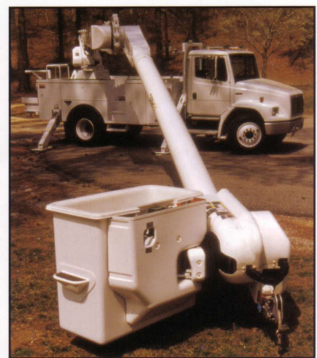
Compact boom tip design allows operator to get close to the work and maneuver in congested areas
