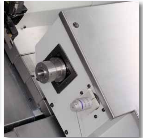
ELITE 27 MS sub spindle.
