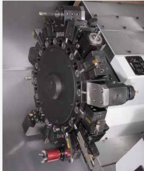
ELITE 27 16-station VDI 25 top plate.
