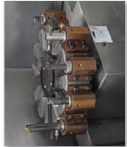
Standard 12-station turret top plate permits very rigid tool positioning
