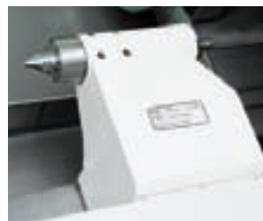
Fully-programmable MT No. 4 Tailstock (SV 150 & SV 200)
