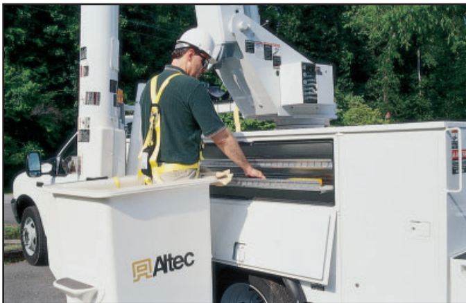
Altec L37M offers easy body compartment access from the platform.
